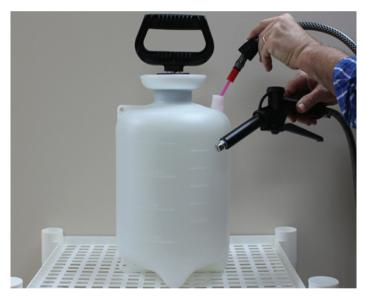
2. Remove the pink drop tube from the red terminus. Insert a paper clip, needle or other piece of metal through both air intake holes in the red terminus to remove debris.
